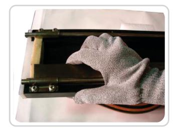
Quick clamping system by means of eccentric bar change of blade aboard deck.
