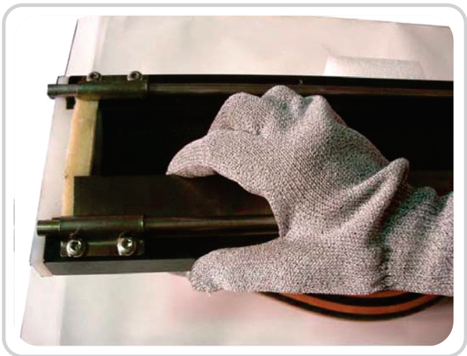
Quick clamping system by means of eccentric bar change of blade aboard deck.
